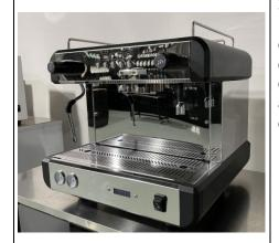
material: stainless stelvoltage(V):220 50Hzpower(W): 2400pump: Italian rotary pump pressure: 9barcontrol panel: PID control gauge\*2 and independen hot water outletExtraction fileter: 58mmbolier: 6L filter holder: 2 water connection: Dierect water connection with rotary pump-conncet with Barreled watercolor: black, white and red accessories: handle\*2(dual+ signle), user manual, inlet pipe, outlet pipe, brush, cleaning gasket
